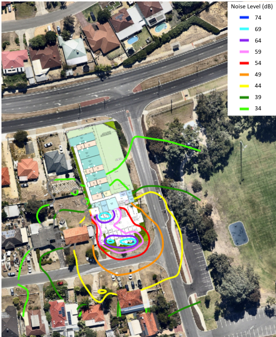
Figure 5: Environmental noise emission prediction night-time ( L_{Amax} ) at 1.5 m above ground level (Assigned Level = 49 dB)
