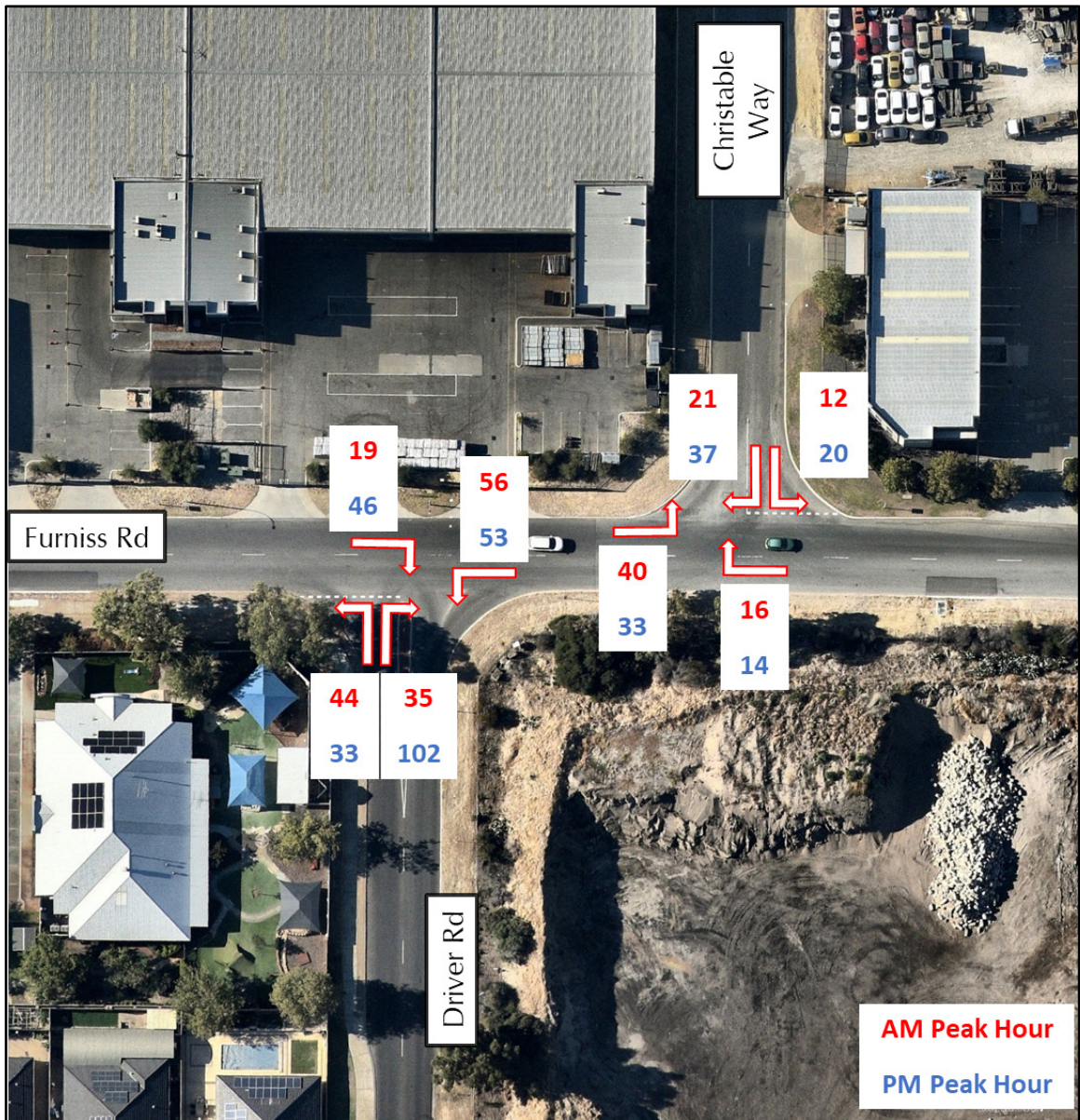
Figure 8: AM/ PM peak hour turn counts at Furniss Road intersections with Driver Road and Christable Way
