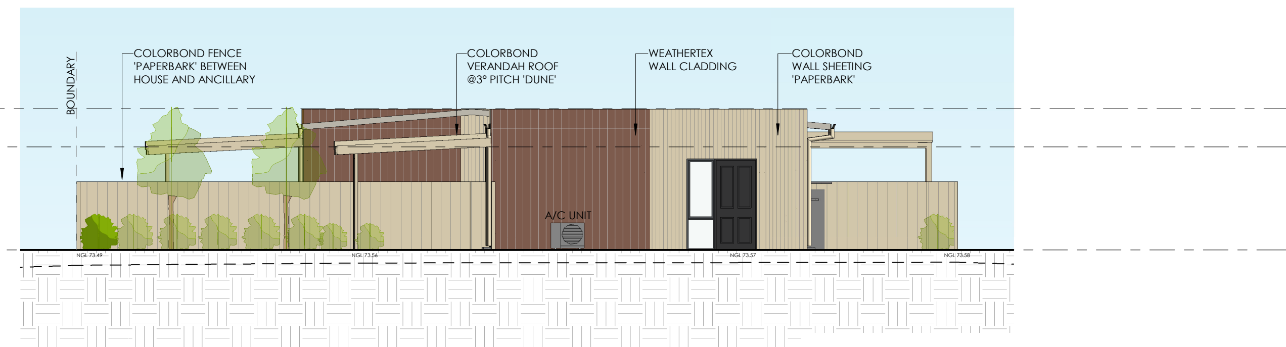
3 WEST ELEVATION DA-02 1 : 100
