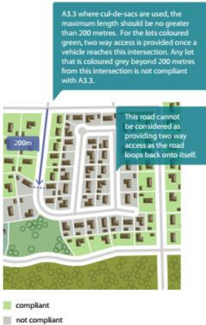
Figure 21: Example of compliant and non-compliant two-way
