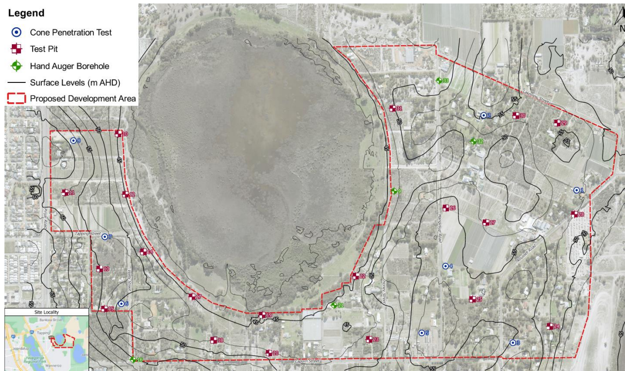
Figure 8 – Geotechnical Test Pit Locations (Douglas Partners)
