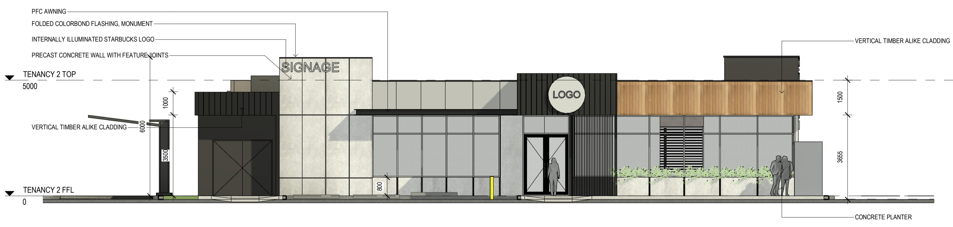
4 TENANCY 2 SOUTH ELEVATION 1: 100
