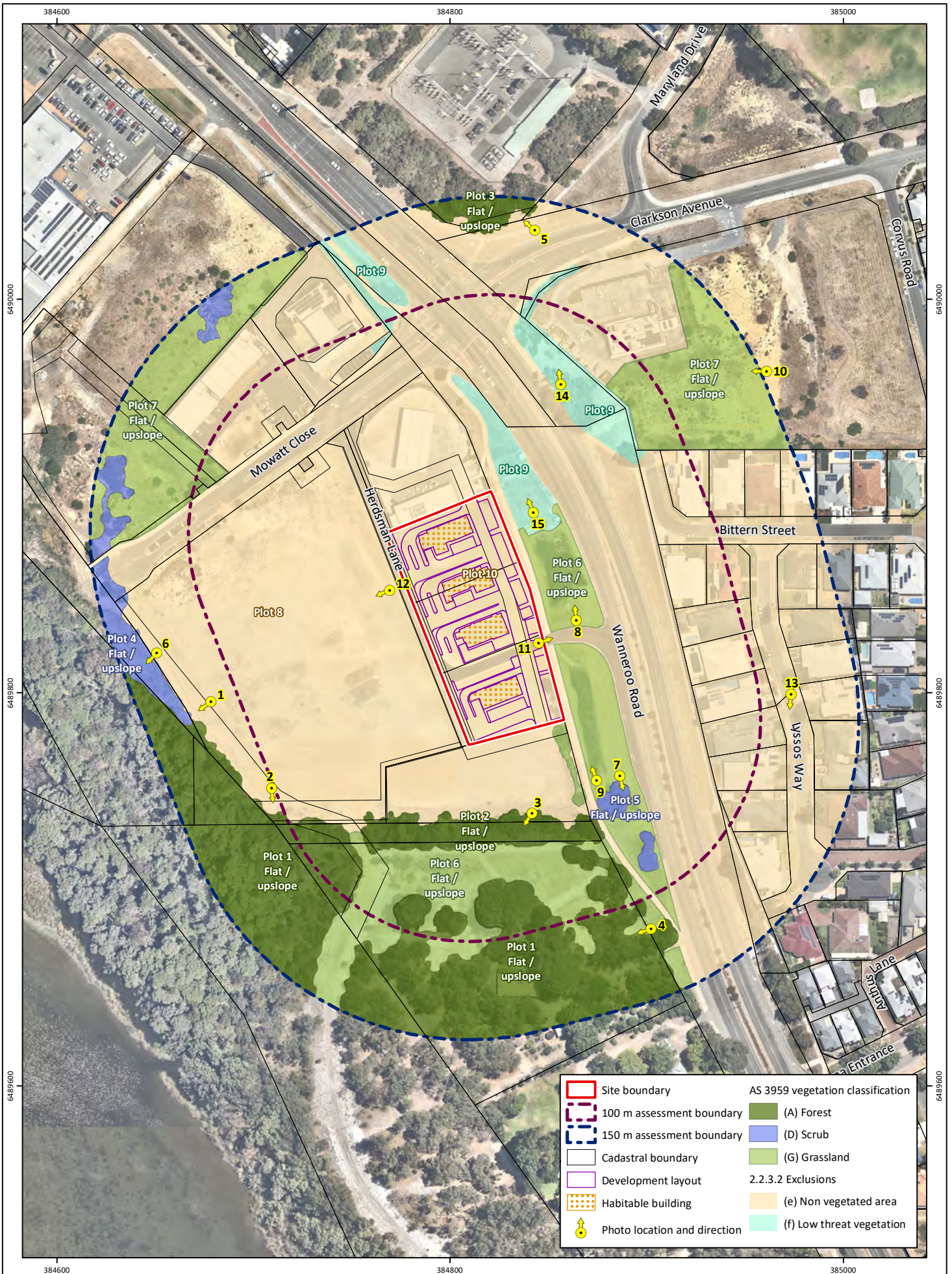
Figure 2: AS 3959 Vegetation Classifications and Effective Slope Project: Bushfire Management Plan Lot 202, Lot 203 and Lot 204, Wanneroo Road, Wanneroo Client: Bella Build & Design WA Pty Ltd
