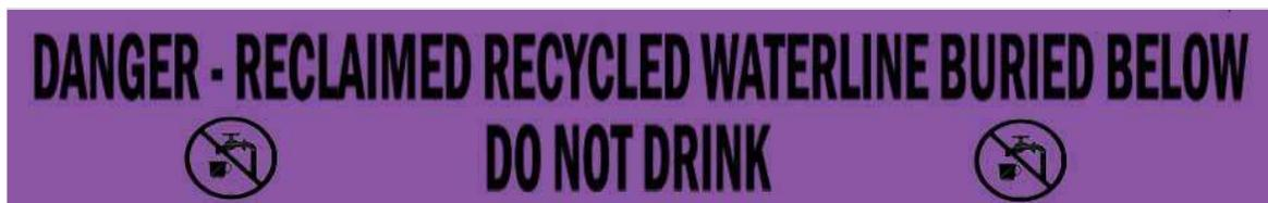
All below ground pipes (including those used for sub-surface irrigation) shall have an identification tape marked in accordance with AS/NZS 3500.1 installed on top of the greywater pipeline, running longitudinally, and fastened to the pipe at not more than 3 m intervals
