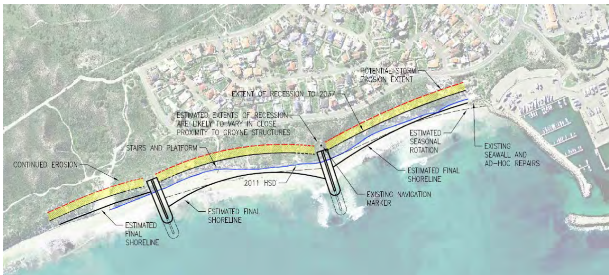
Figure 6.7 - Shoreline Recession & Potential Severe Storm Erosion to 2037
