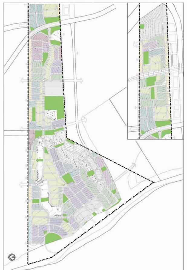
Within the proposed Coastal Village, earthworks would be required to provide development sites with grades of less than 3% to accommodate the mixed land uses within the village. The Structure Plan also encourages alternative building forms including framed and split level housing to better suit existing slopes.
