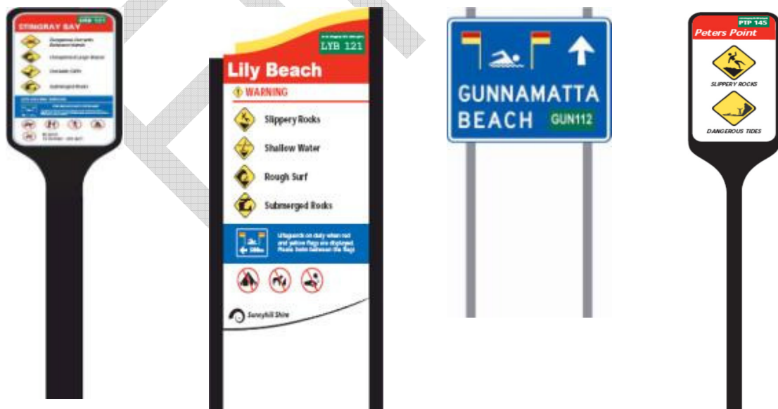
Level 3: Defined Access Type B: 3 or 4 Hazard Symbols
