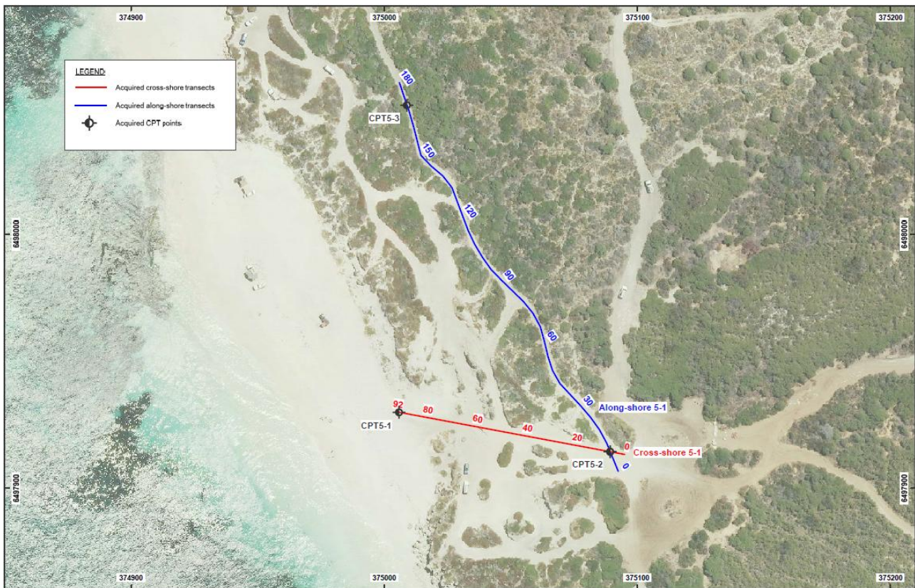
Figure 2-6 Locations of cross-shore (red) and alongshore (blue) transects and CPT pits completed at Site 5 (Northern Area) (GBG Maps 2016)
