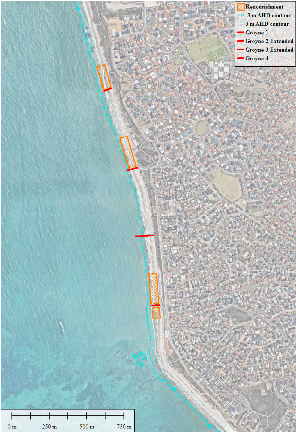
Figure 3-1 MCA2/LITPACK Option 12 from Cardno (2016). Groyne 1 unchanged in length, Groynes 2 and 3 extended. Groyne 4 new structure.
