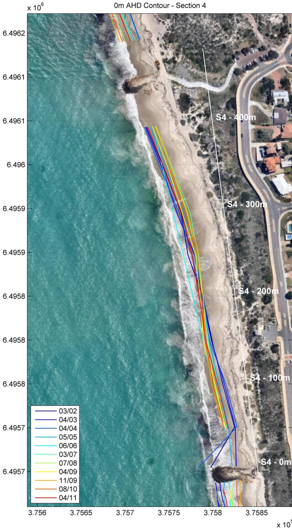
Figure B-4 Plot of 0 m AHD contour line derived from beach survey data for February to November 2014 in Section 4. The white line is the baseline with chainage along this line shown. The aerial photo background is from November 2014.
