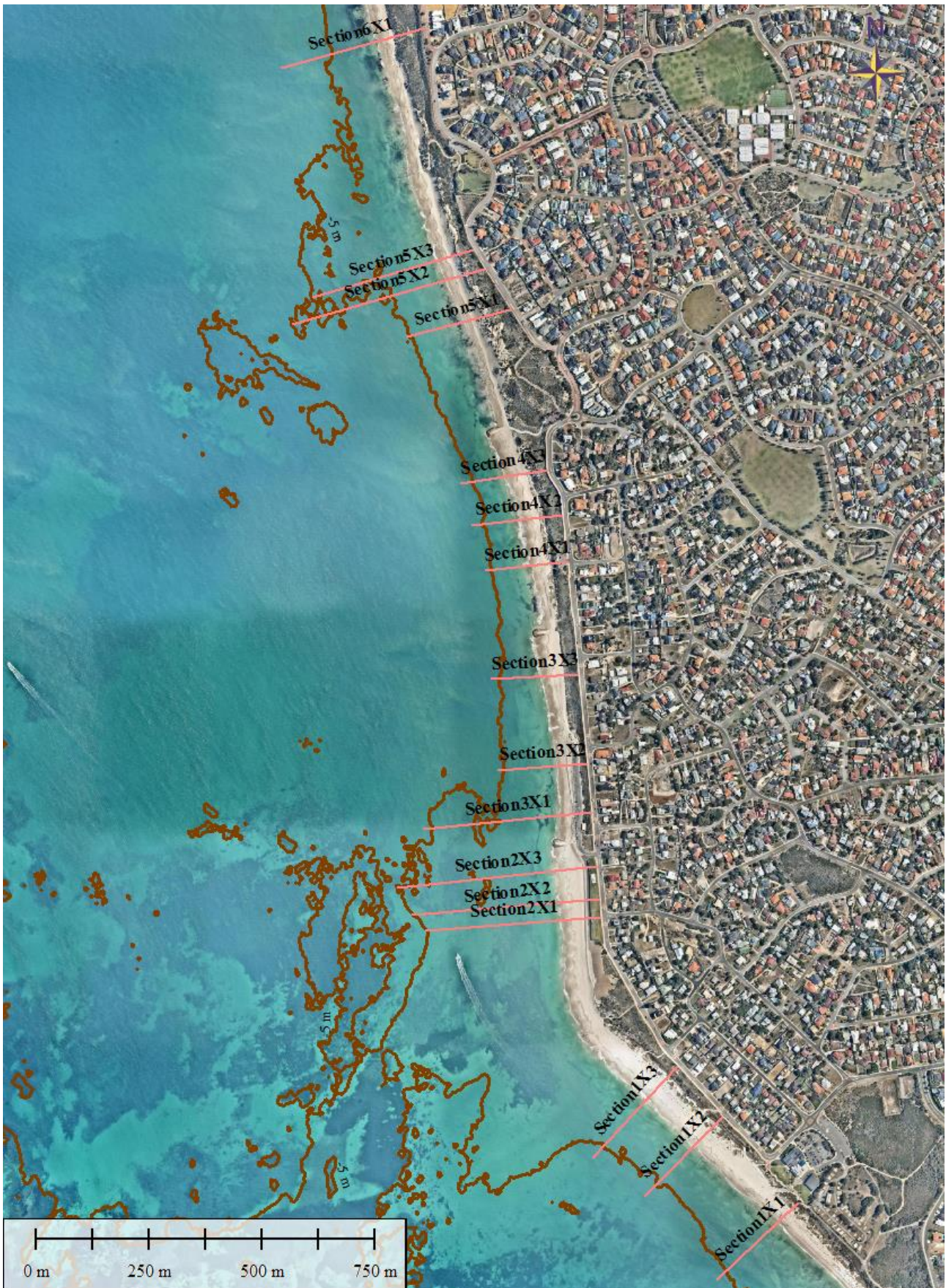
Figure C-8 Profile locations where the XBeach and Delft3D models were assessed.
