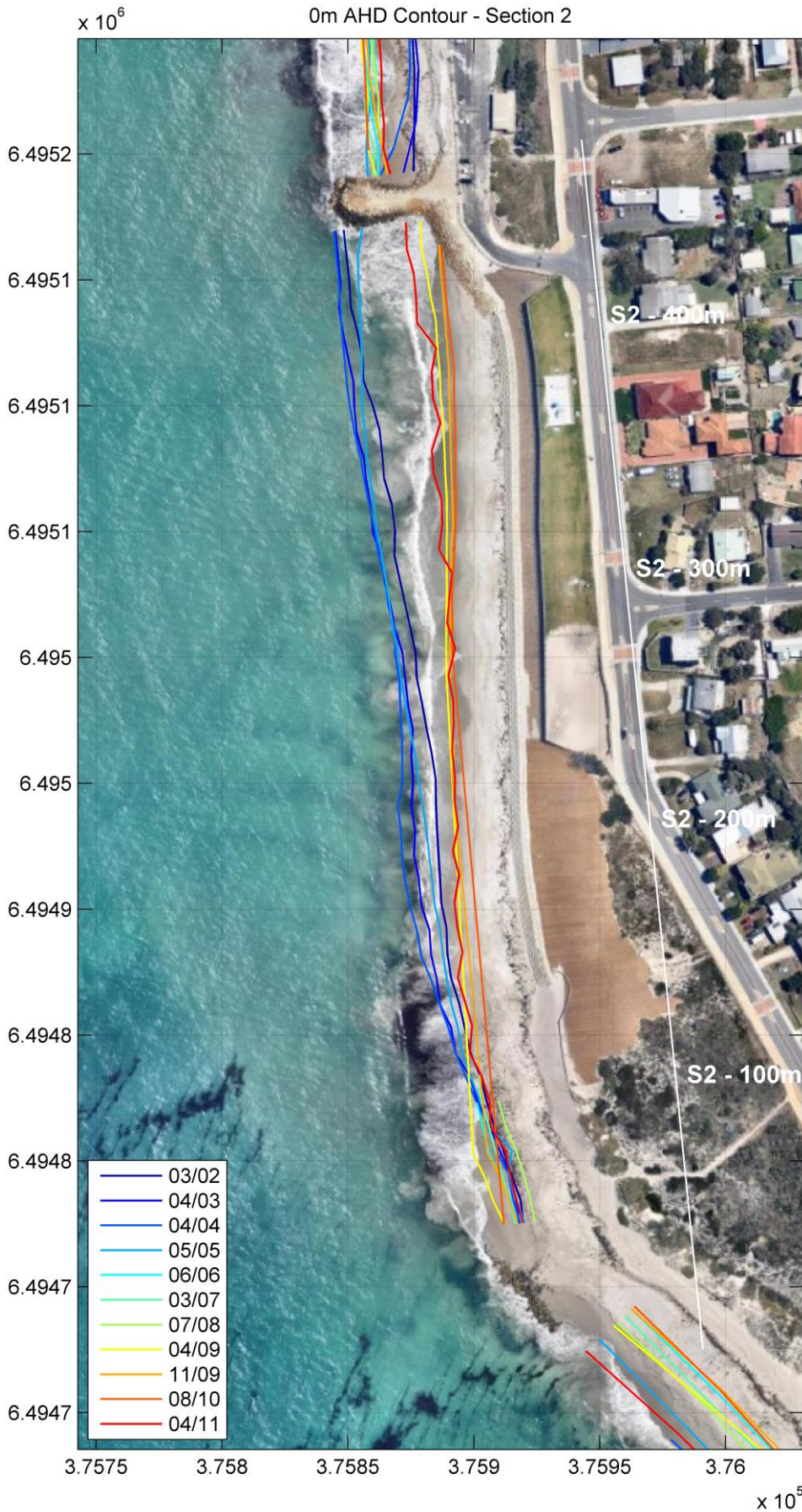
Figure B-2 Plot of 0 m AHD contour line derived from beach survey data for February to November 2014 in Section 2. The white line is the baseline with chainage along this line shown. The aerial photo background is from November 2014.
