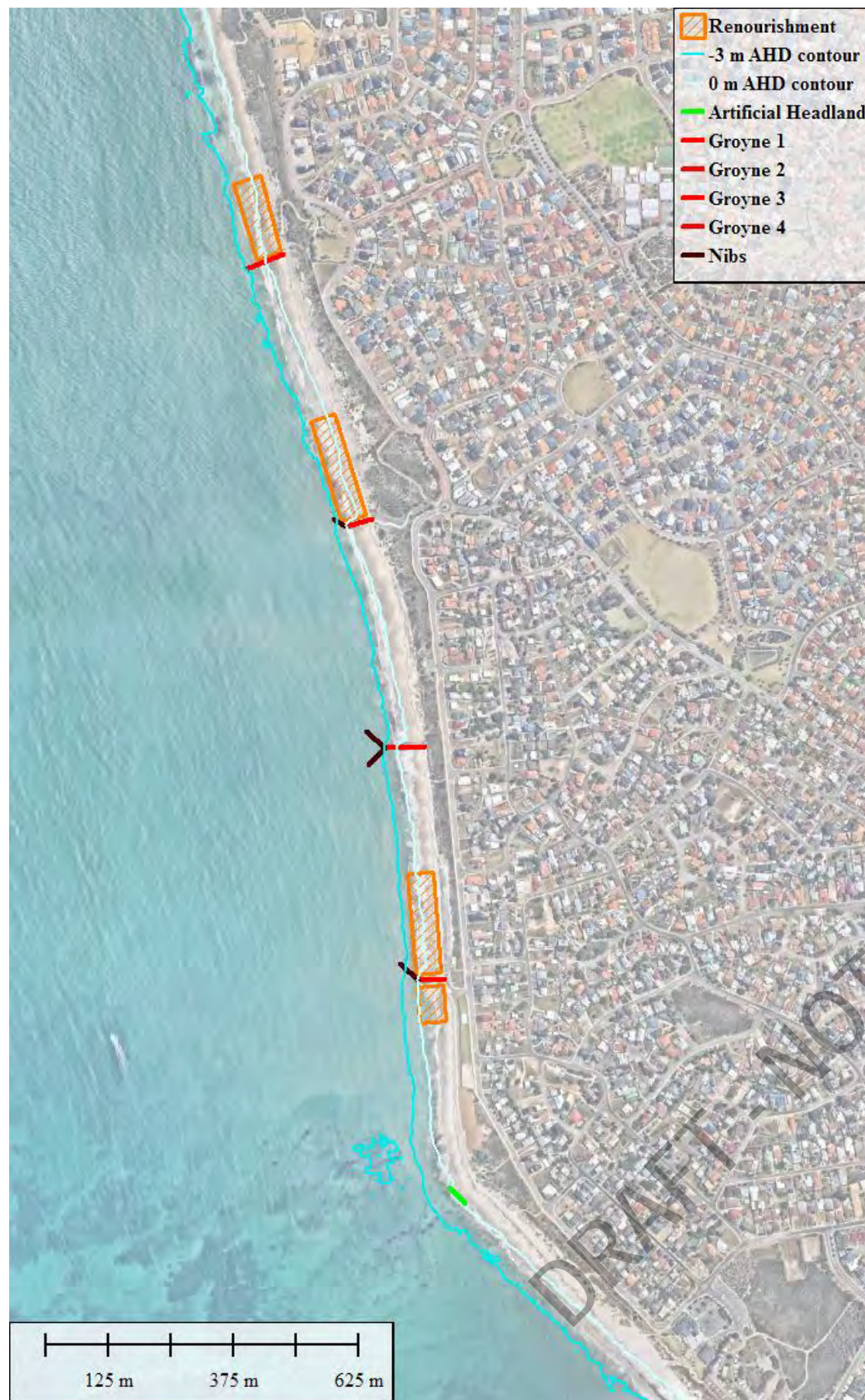
Figure 3-3 Conceptual Layouts for (a) MCA4 and (b). MCA5. Structures shown in green are existing structures; red are new / adapted structures; dark brown are breakwater nibs
