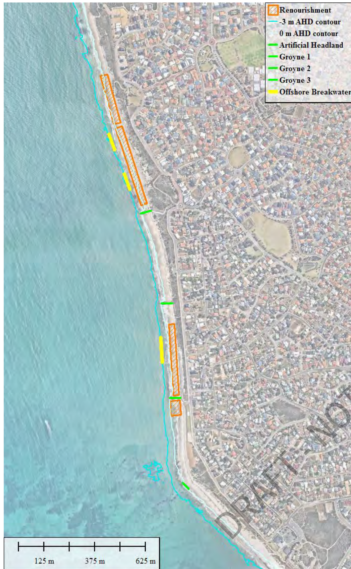
Figure 3-1 Conceptual Layouts for (a) MCA1 and (b) MCA2. Structures shown in green are existing structures; yellow are offshore breakwaters; red are new / adapted structures
