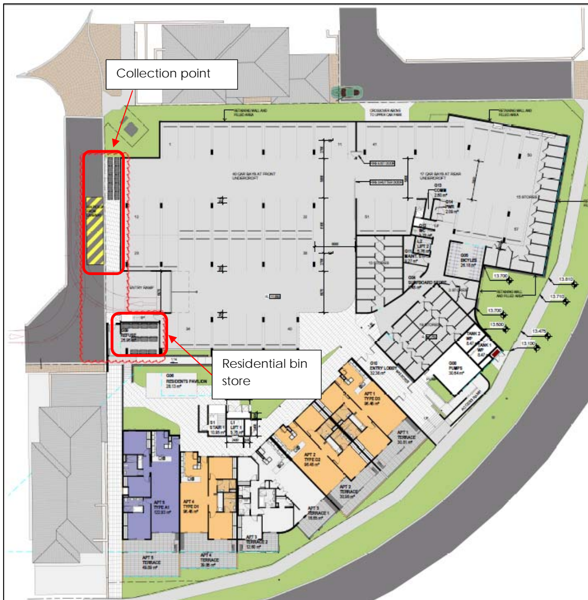
Figure 1: Ground floor plan showing the residential bin store and collection point
