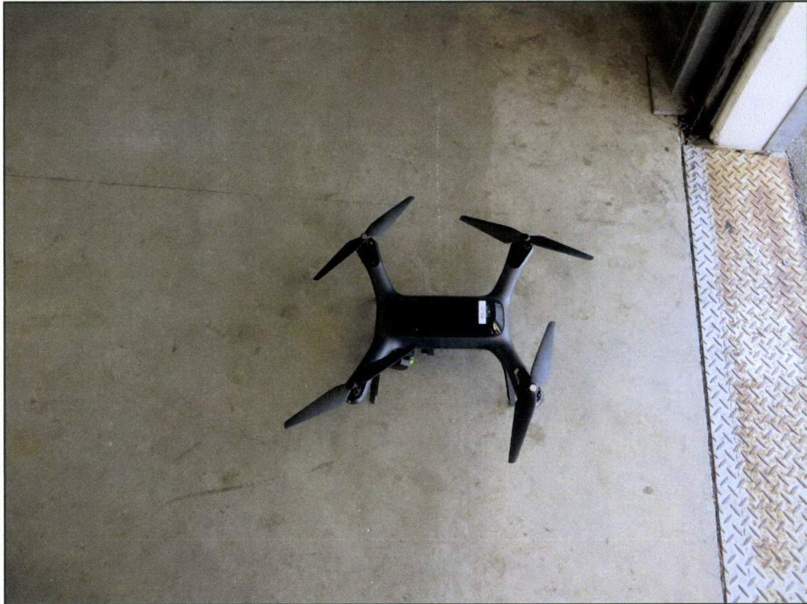
Figure 14 The remote-controlled device used to establish an accurate height datum
