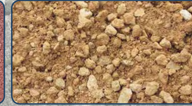
Compacted crushed limestone
