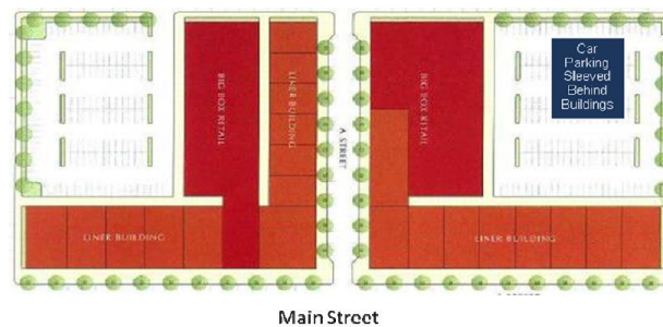
Car parking is to be sleeved behind buildings in a reciprocal lot.
