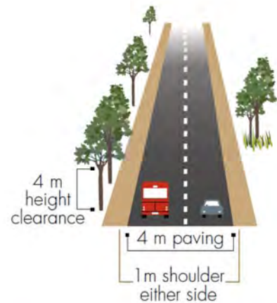
Figure 19: Minimum design requirements for a public road
