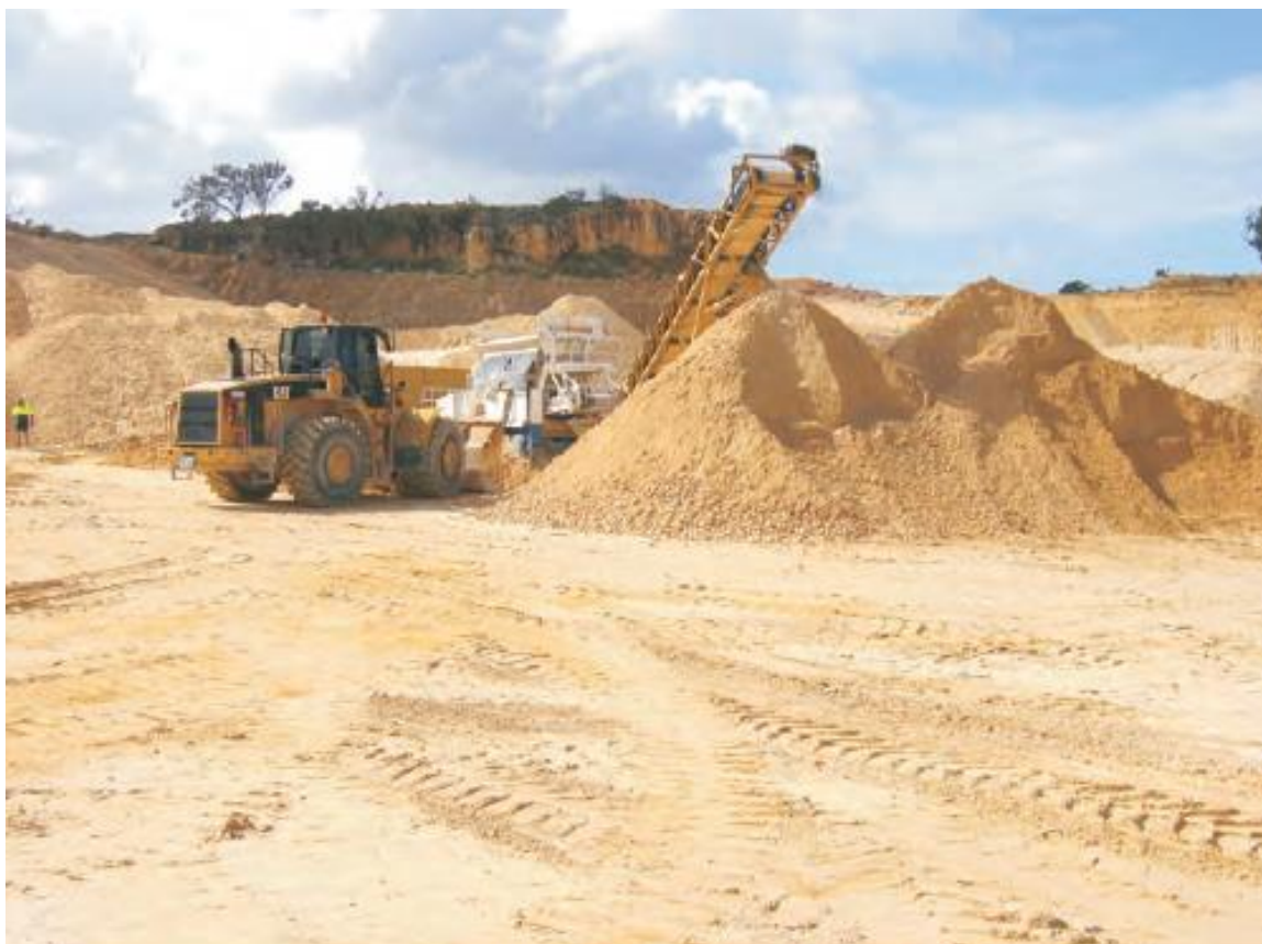
Loader feeding a working crusher
