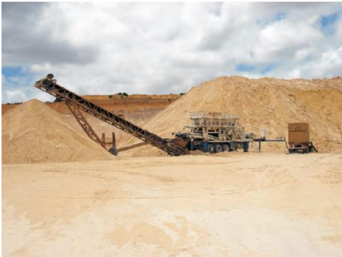
Limestone crushing plant
