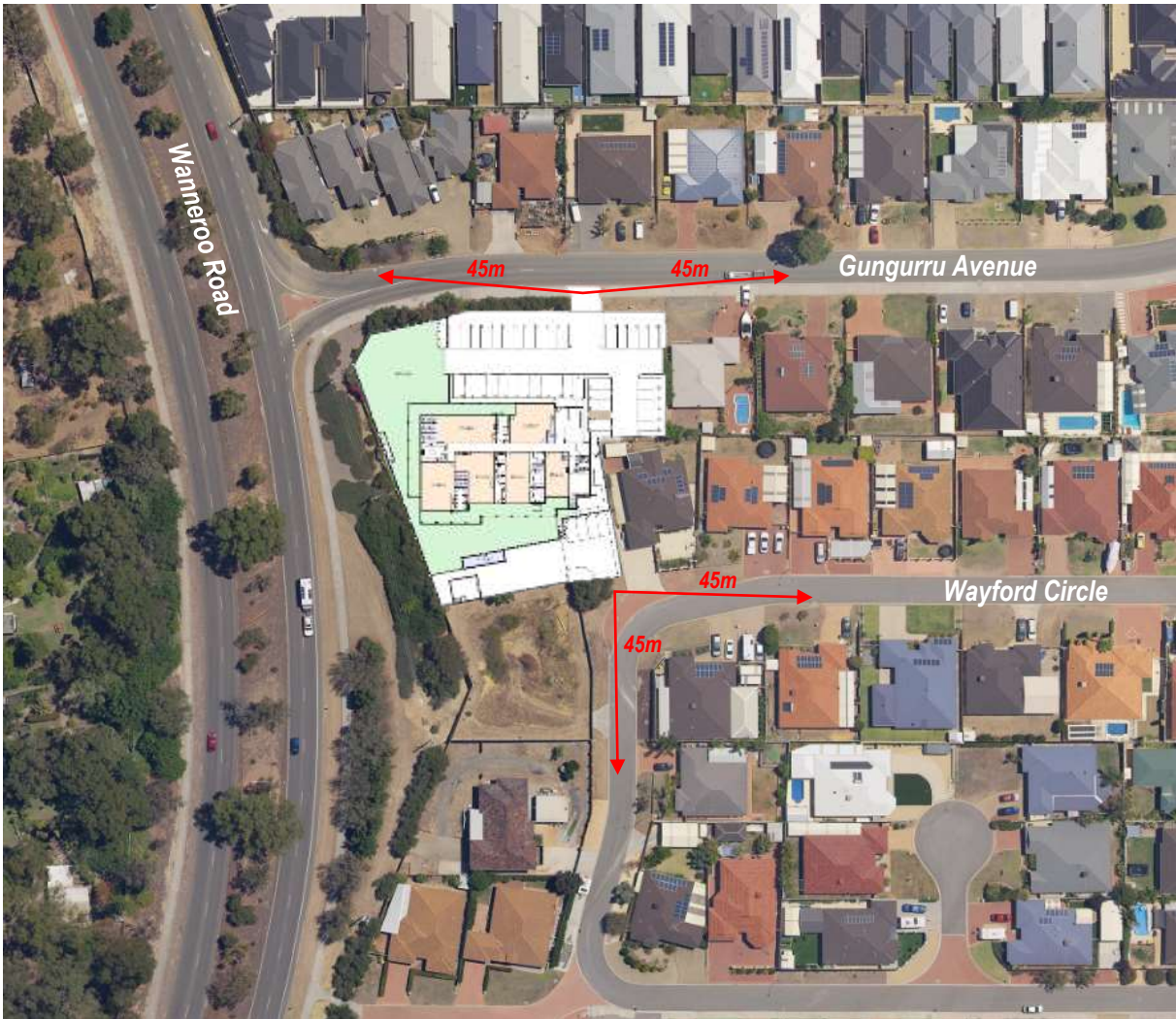
Figure 9: Access Sight Distance
