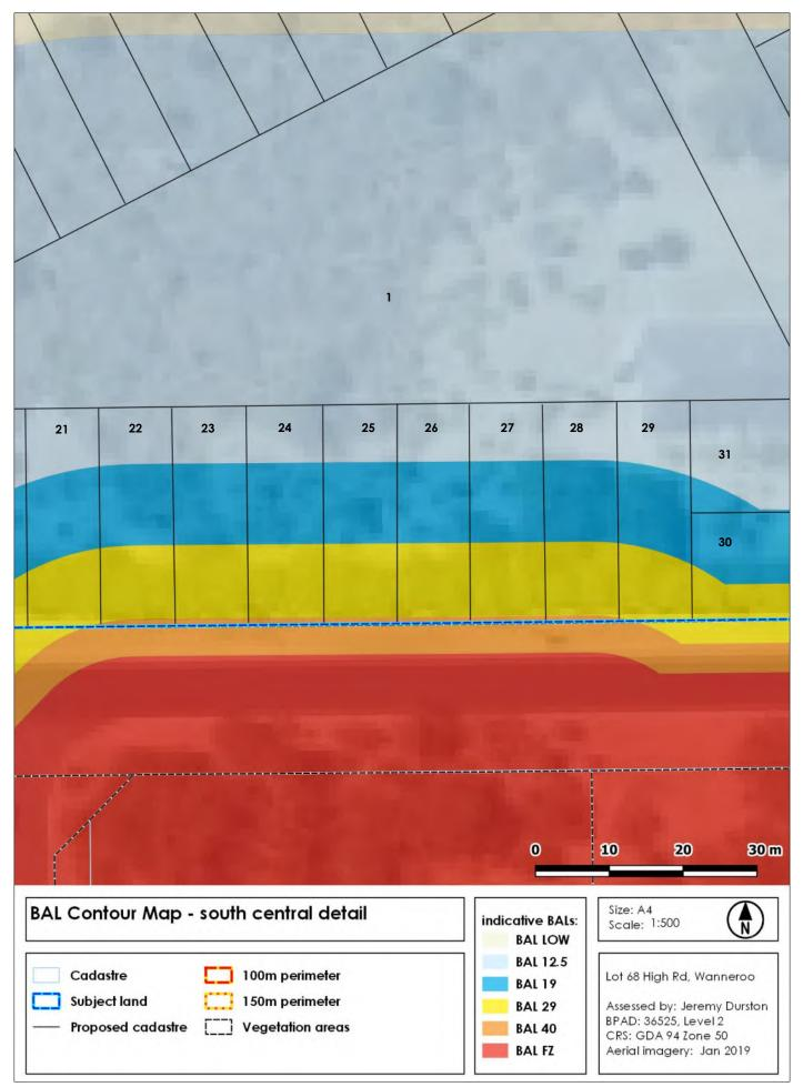
Figure 5F: BAL Contour Map, central-southern section detail
