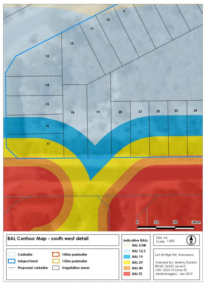
Figure 5E: BAL Contour Map, south-western section detail
