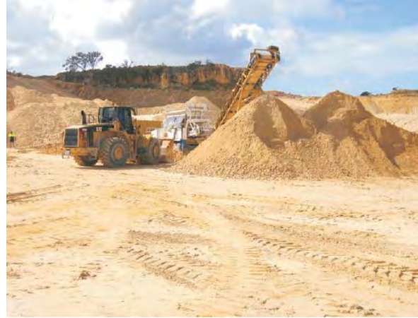
Loader feeding a working crusher
