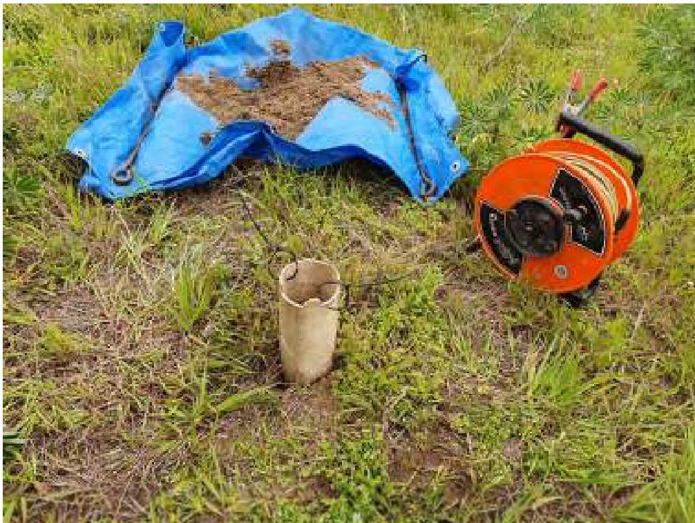
Photograph 2: IT04 (Unit 1a SAND FILL) – Inverse auger hole test setup
