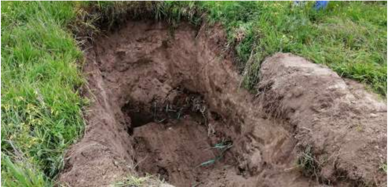
Photograph 5: Example test pit for infiltration testing in Unit 1B (Uncontrolled FILL) material – prior to water addition
