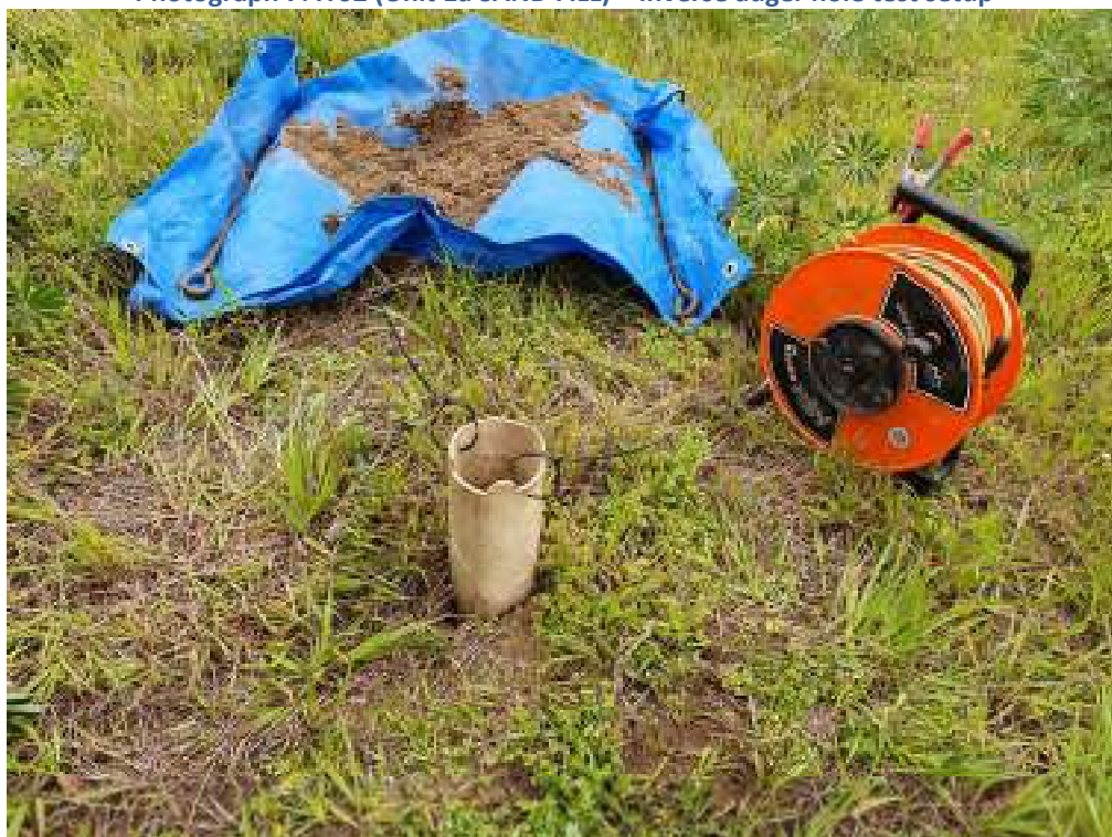
Photograph 8: IT04 (Unit 1a SAND FILL) – Inverse auger hole test setup
