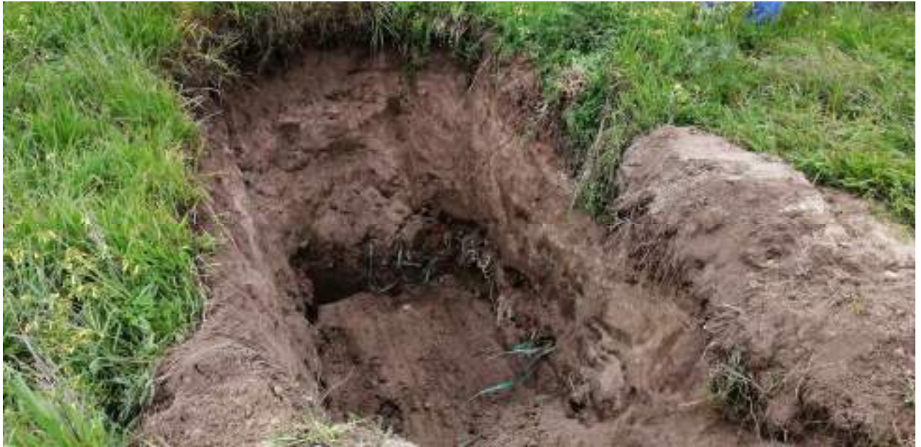
Photograph 11: Example test pit for infiltration testing in Unit 1B (Uncontrolled FILL) material – prior to water addition
