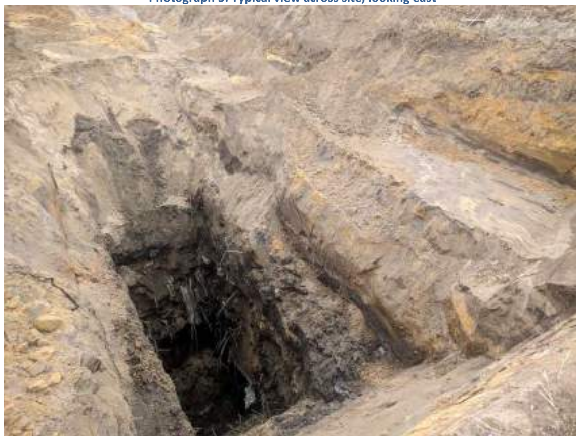
Photograph 6: Typical profile of sand fill overlying uncontrolled fill including rubbish
