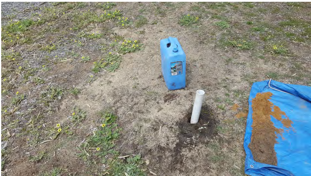
Photograph 8: Typical view of infiltration test set up.
