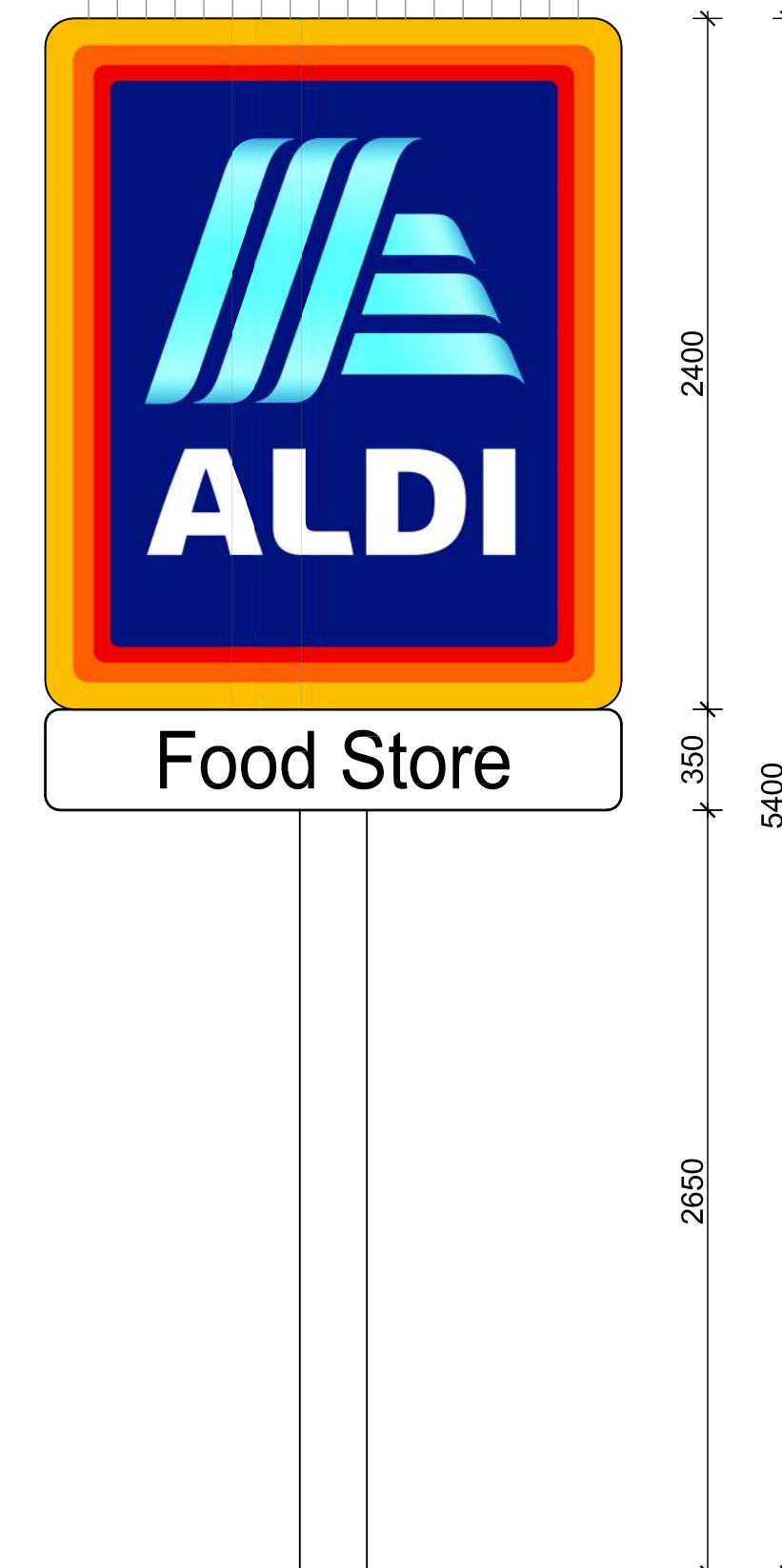
4 ALDI PYLON SIGN SIGN 1 SCALE 1:25
