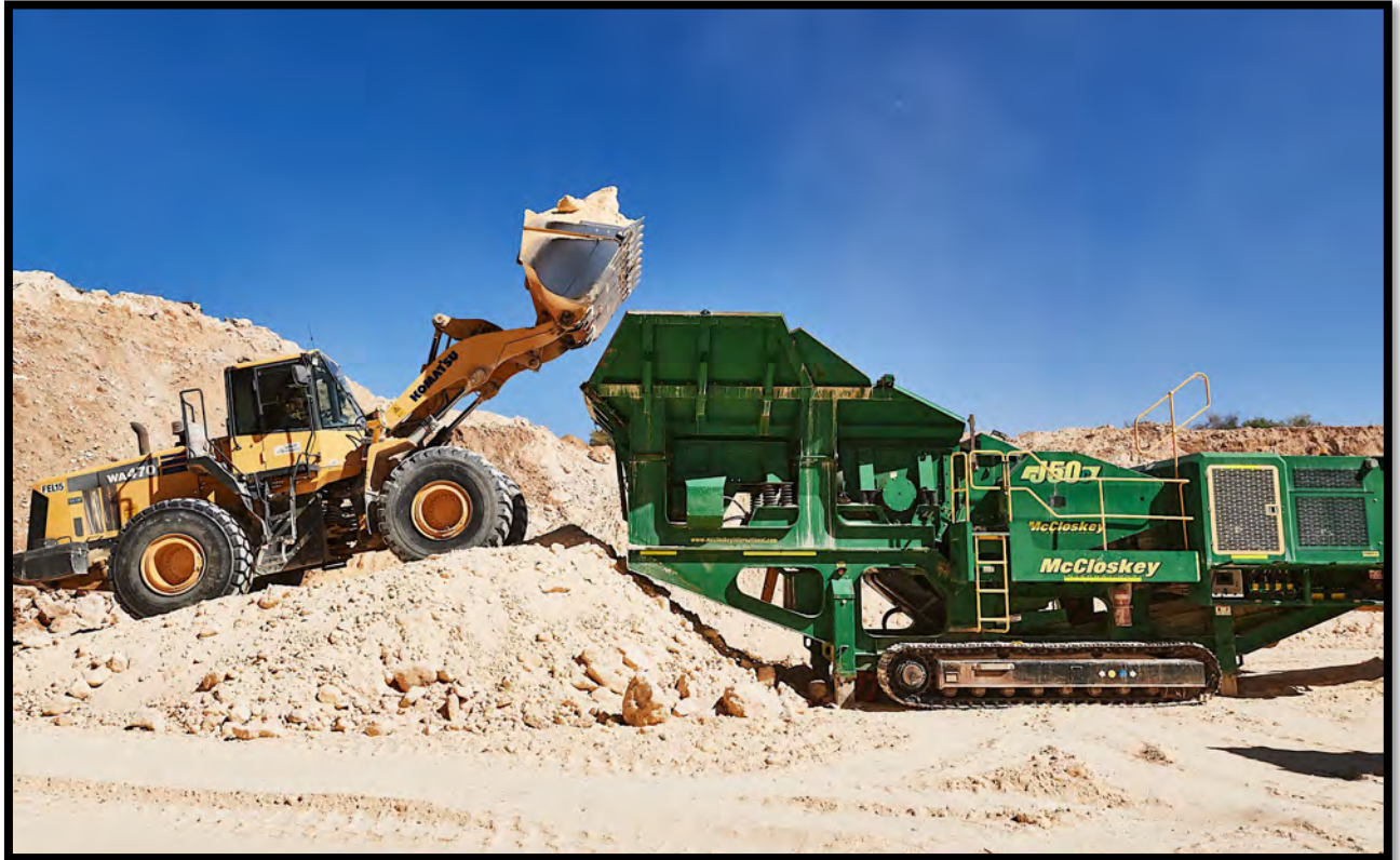
Figure 9: Feeding limestone to a crushing plant
