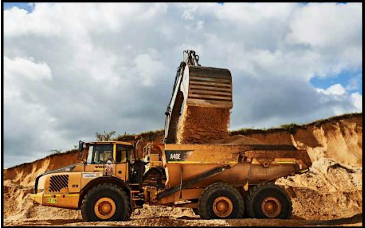
Figure 7: Loading an internal haul truck
