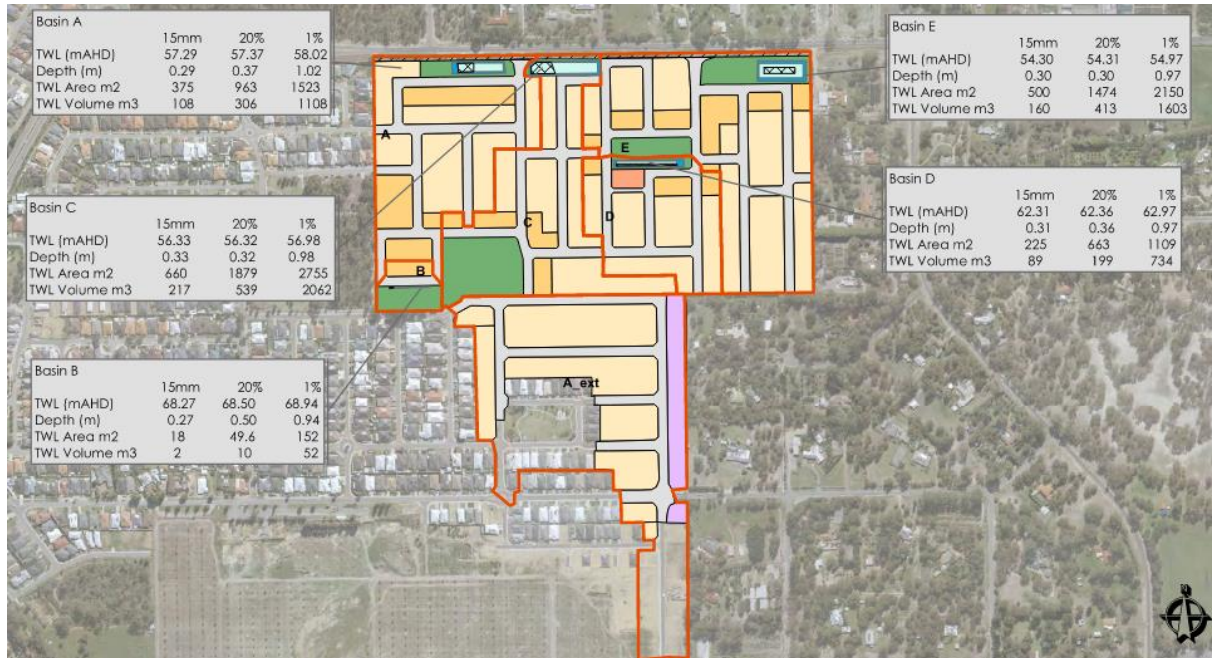
Figure 4 – Proposed drainage catchments and basins (Hyd2o, August 2020)
