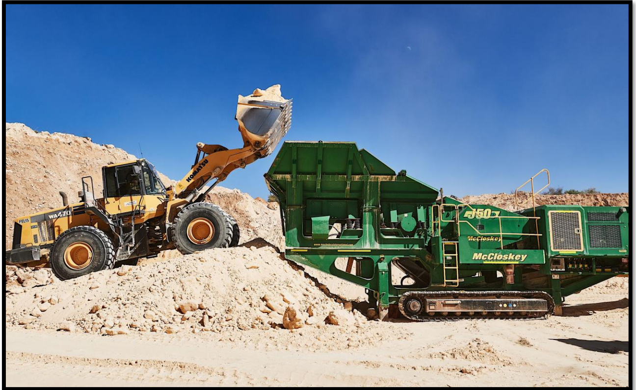
Figure 9: Feeding limestone to a crushing plant
