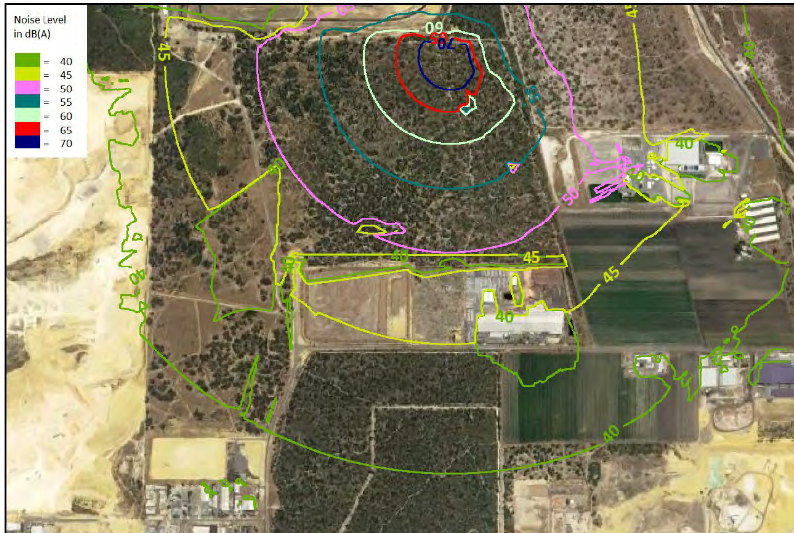
Figure 11: Worst-case noise contours for scenario 8 – mining at the north-eastern part of stage 5 pit.
