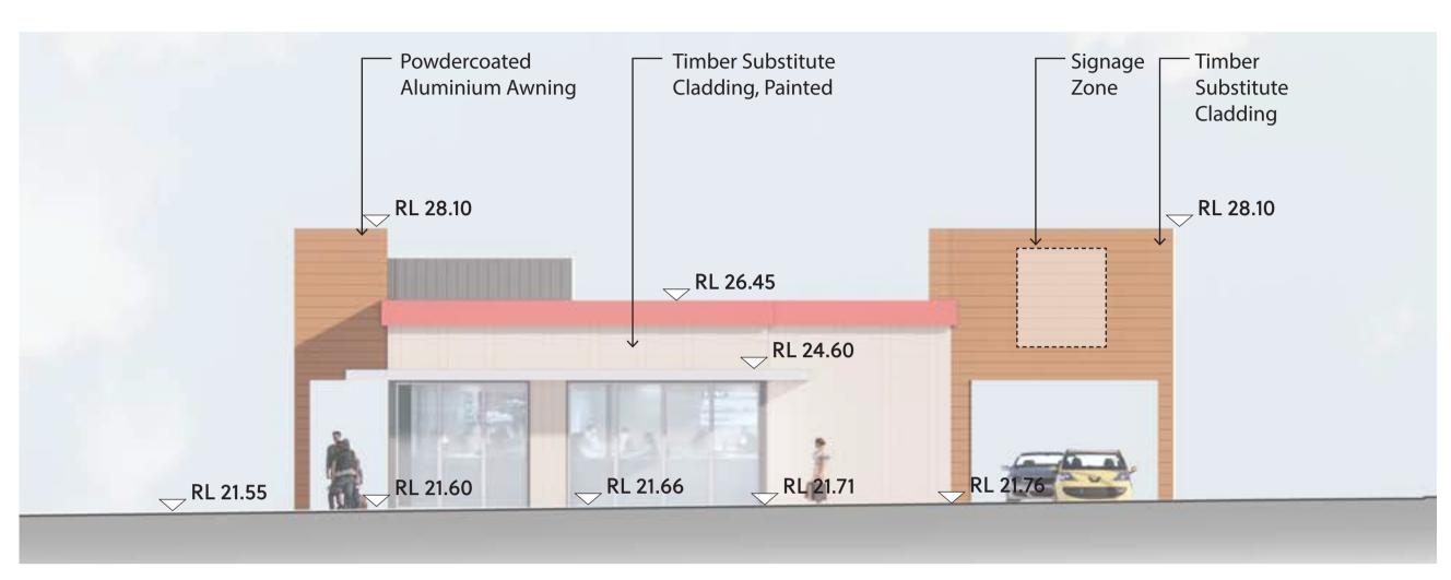
Timber Substitute Signage Zone Powdercoated Aluminium Cladding, Painted Awning RL 28.10 \_\_\_ RL 26.45 \_\_\_ RL 21.48
