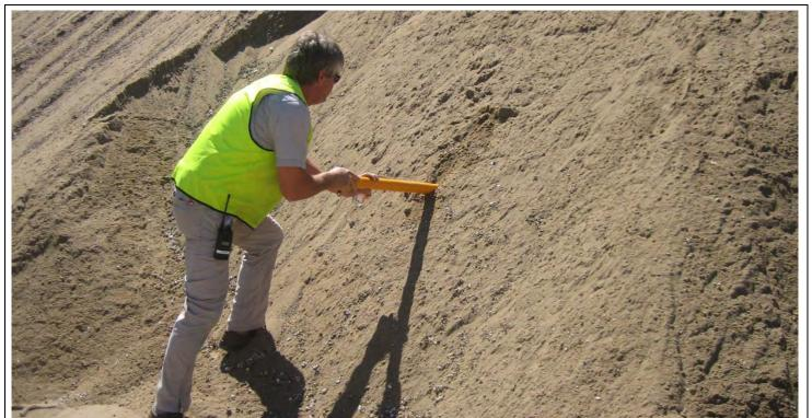
Photograph One: Hollow sampling tube is inserted into the base of the stockpile (approx. 500-750mm)
