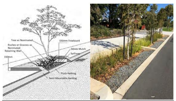
Figure 13: Typical roadside tree pit or raingarden
