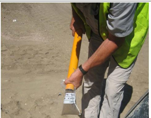
Photograph Three: Soil is transferred directly from sampling tube into a plastic bag for asbestos analysis
