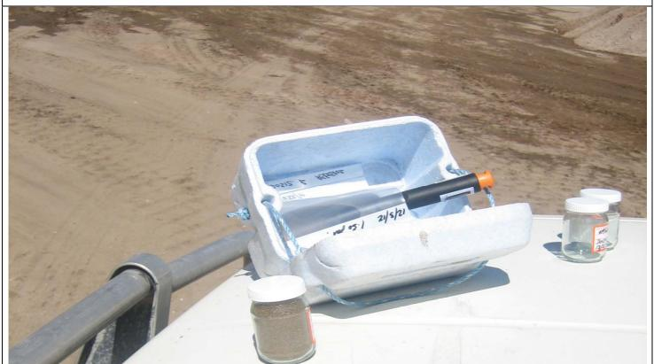
**Photograph Four:** Soil samples are placed directly into an esky for transport to the laboratory
