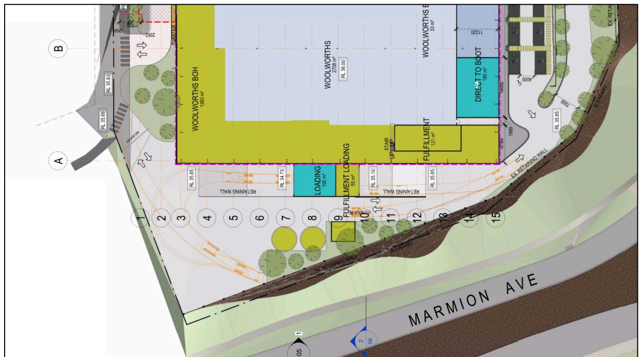
Figure 10 Delivery Vehicle Swept Path
