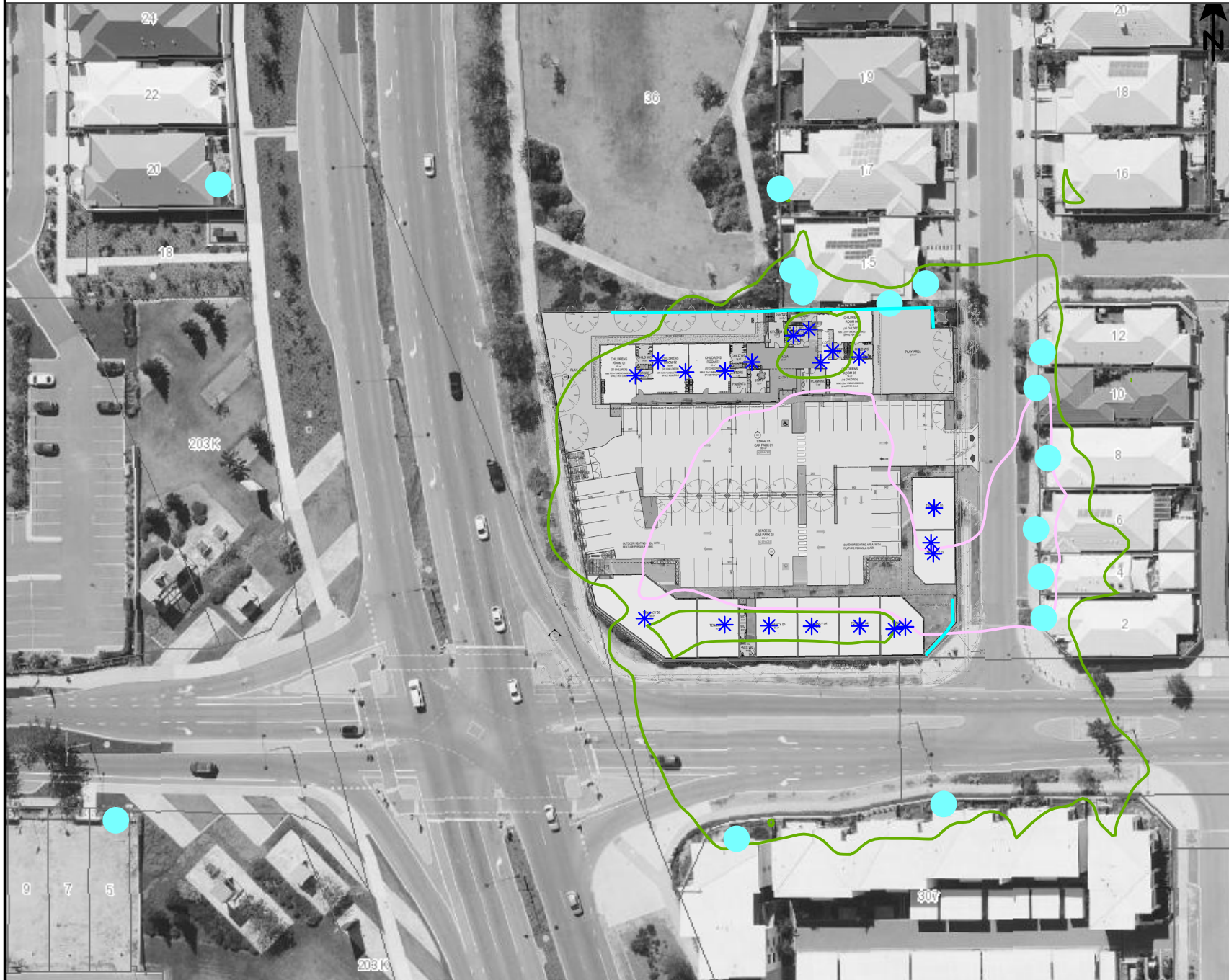
Figure 4-2 Mechanical Plant Noise, Night Time, dB LA10
