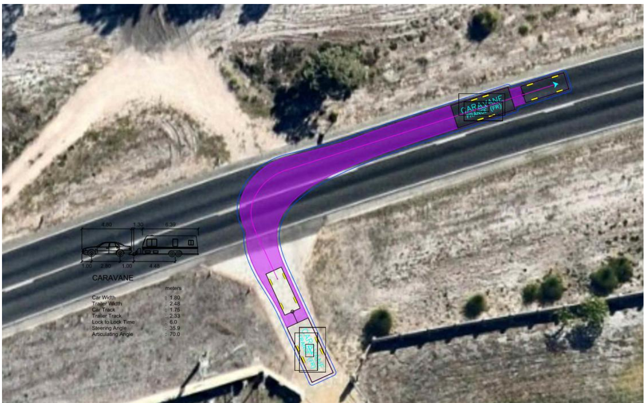
Figure 3-8 Swept Path – RIGHT OUT
