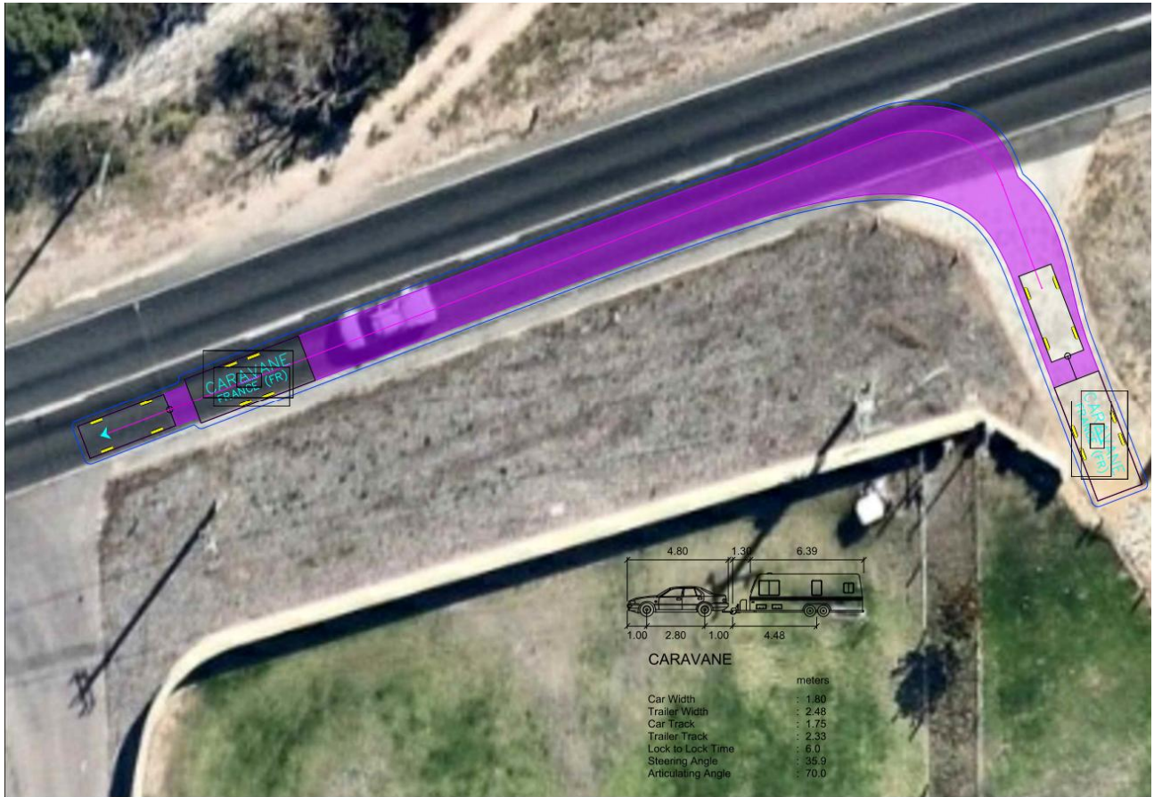
Figure 3-8 Swept Path – RIGHT OUT
