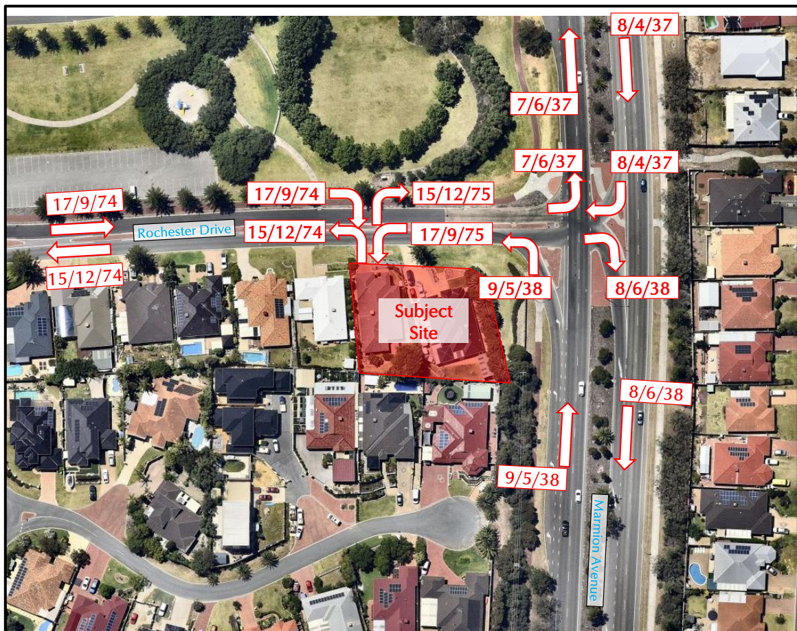
Figure 4: Estimated traffic movements for the subject site AM Peak/PM Peak/Total daily trips
