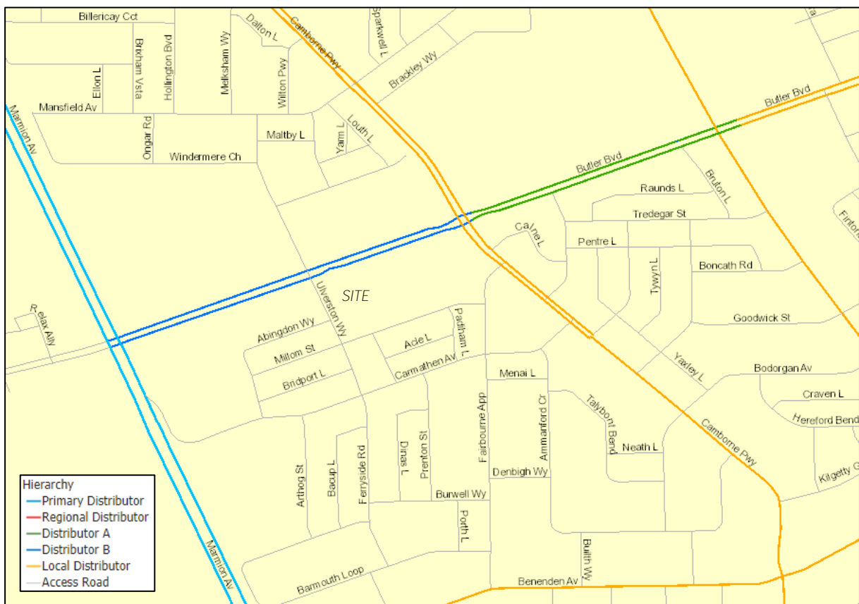
Figure 4: Existing Road Network Hierarchy
