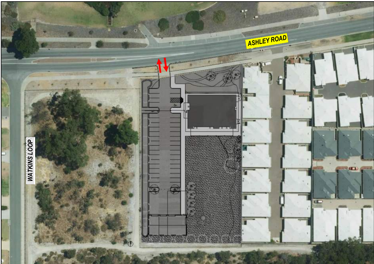
Figure 7: Vehicle Access Arrangement
