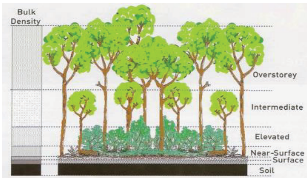
Plate 3: The five fuel layers in a forest environment that could be associated with fire behaviour (Gould et al. 2007)
