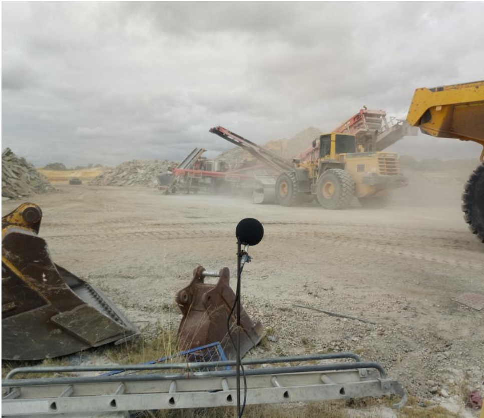
Figure 3-1 Noise Monitoring Logger At Pit Area
