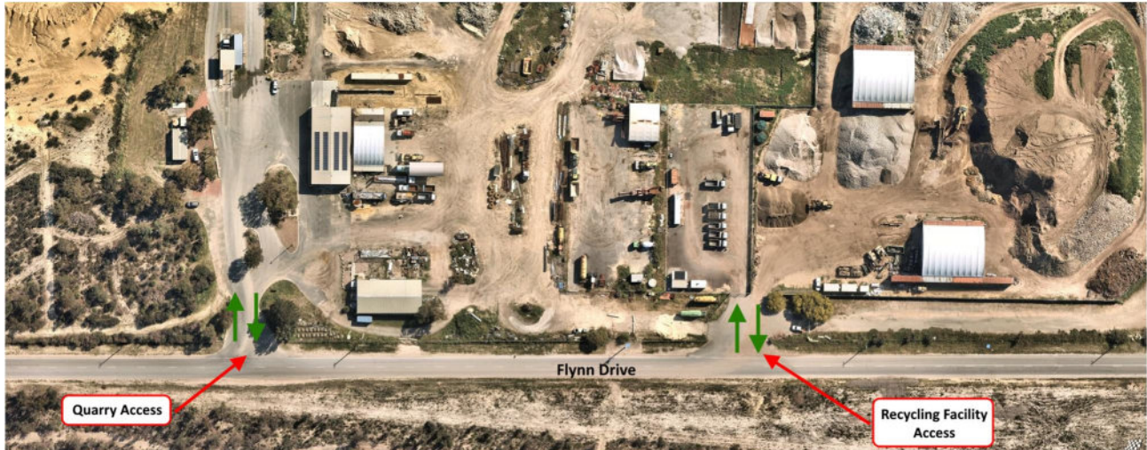
Figure 2-3 Existing Access Arrangement of Lot 901
