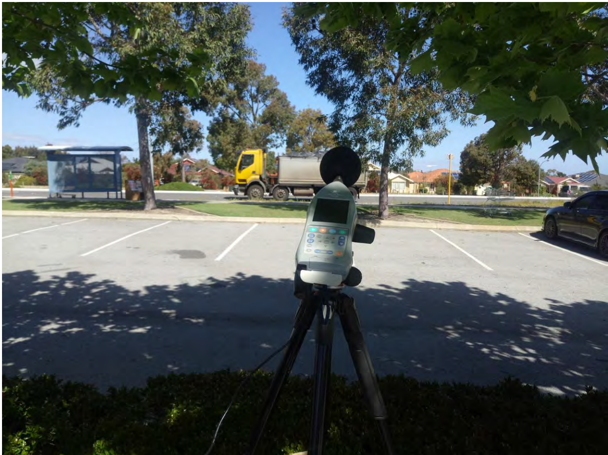
Figure 3-1 Sound Level Meter on Site
