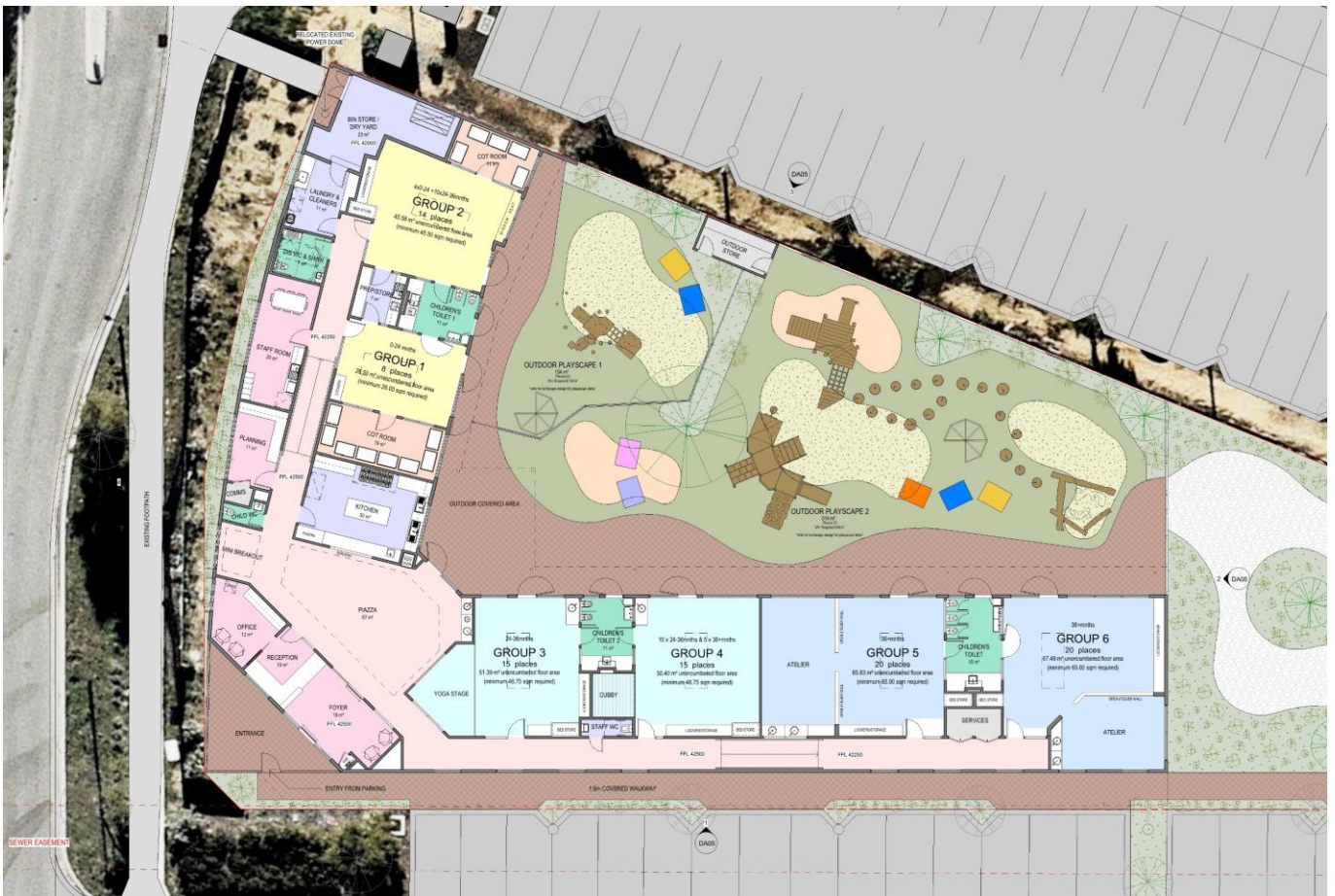
Figure 5 Site floor plan for the proposed Butler Childcare Centre (source: Peter Hobbs Architects, 2022)
