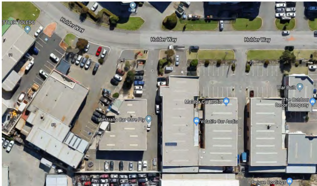
Figure 4-19 Example of inefficient, irregular lot configuration
