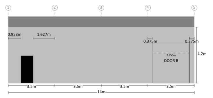
Measurements are from the outside of end girts (end bays) and/or centre of columns (mid bays) to inside of component opening size.
