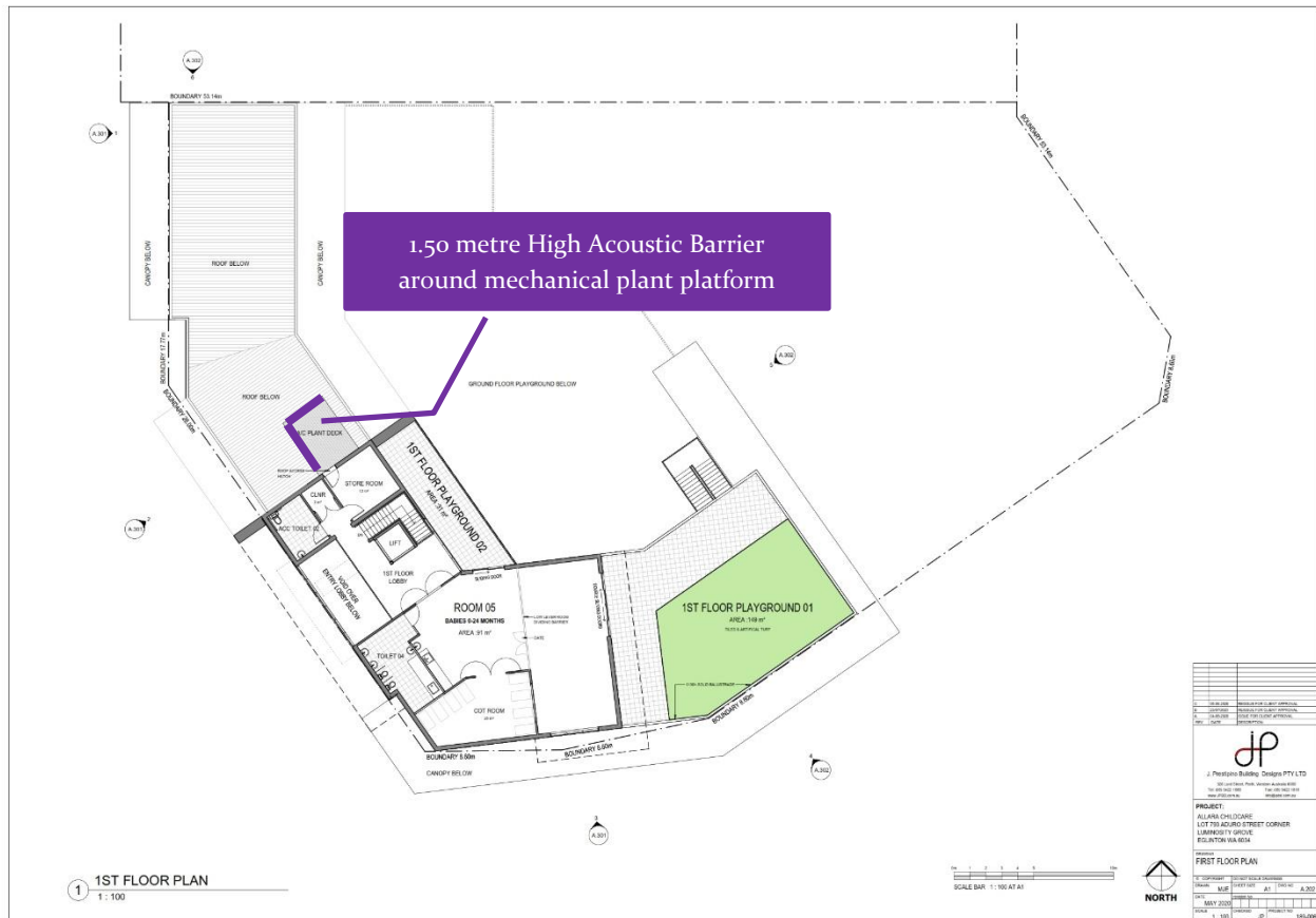
Figure 7.1: Acoustic Barrier Location and Height
