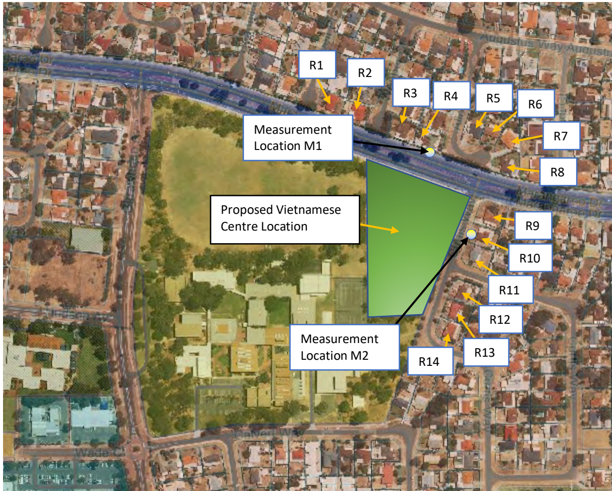
Figure 1: Aerial imagery of proposed site, nearest noise sensitive receivers and measurement location
