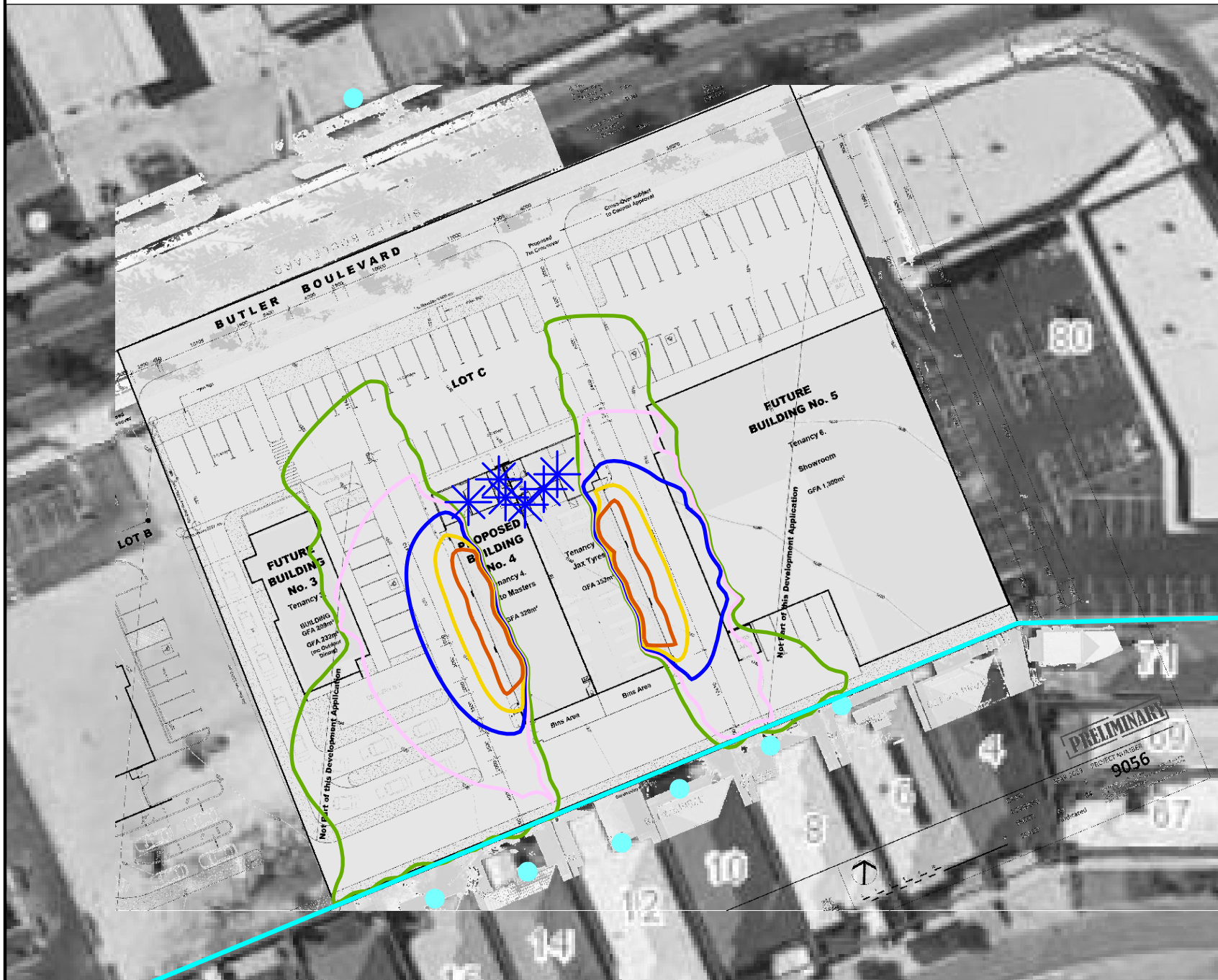
Figure 4-1 L_{A10} Normal Operations Noise Contour Plot (1.4m AGL), dB
