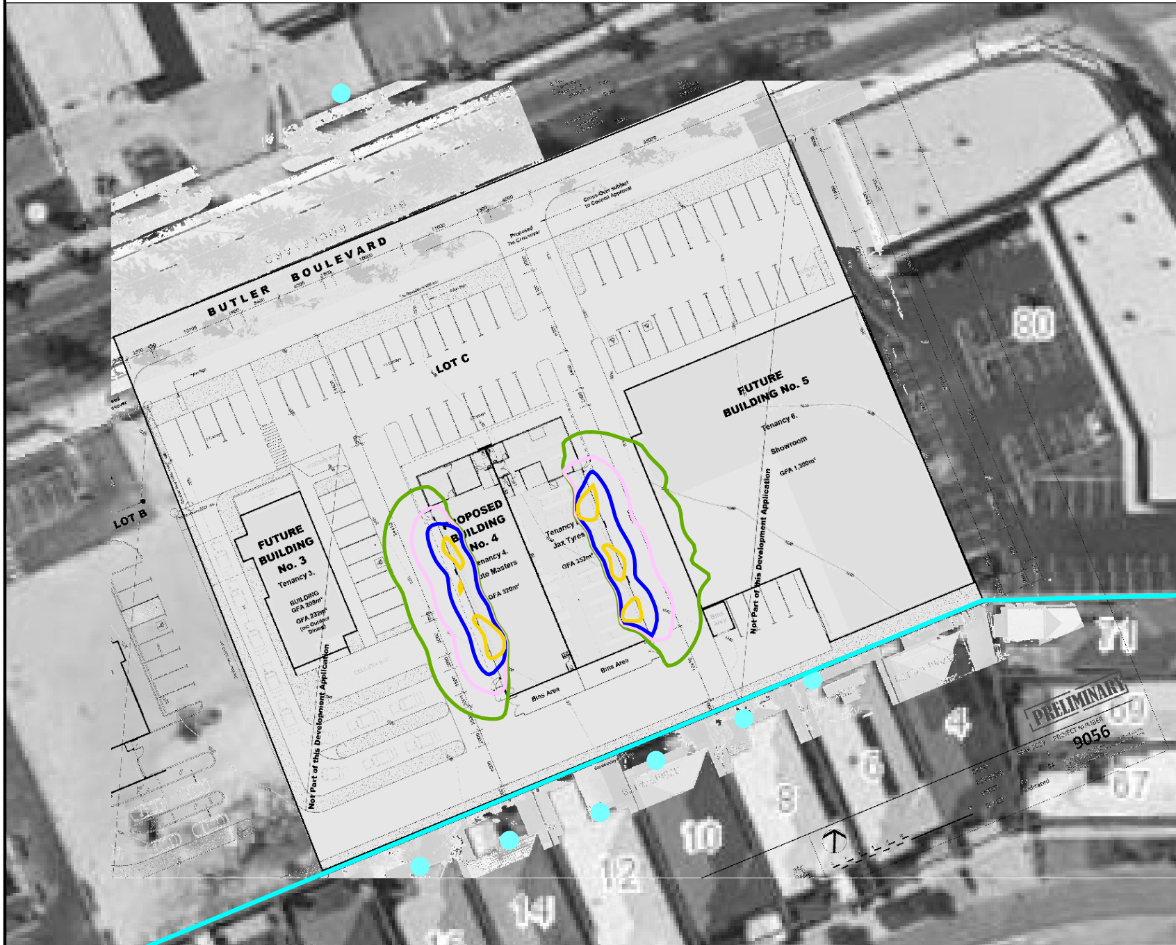
Figure 4-2 L_{Amax} Normal Operations Noise Contour Plot (1.4m AGL), dB
