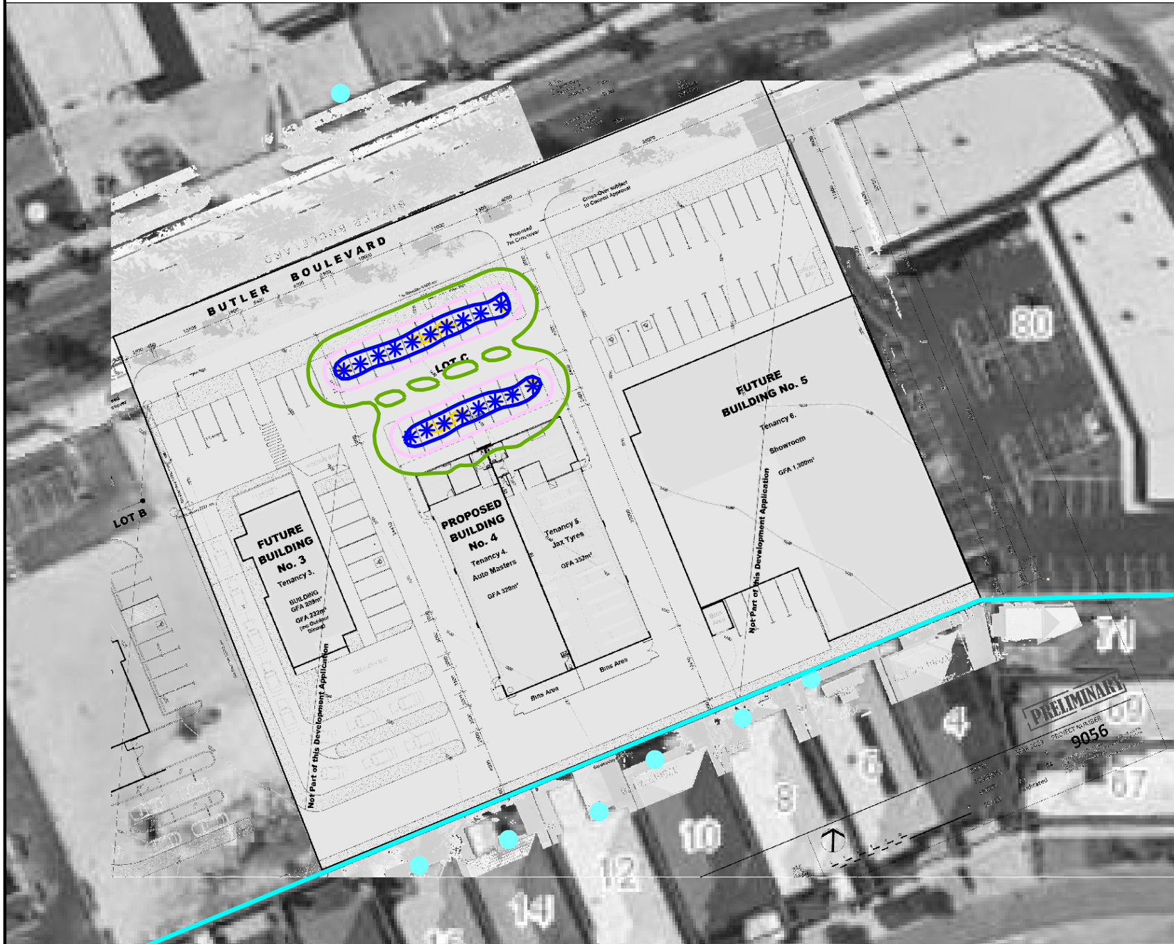
Figure 4-3 L_{Amax} Car Door Noise Contour Plot (1.4m AGL), dB
