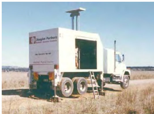
Figure 2: Purpose built CPT rig
