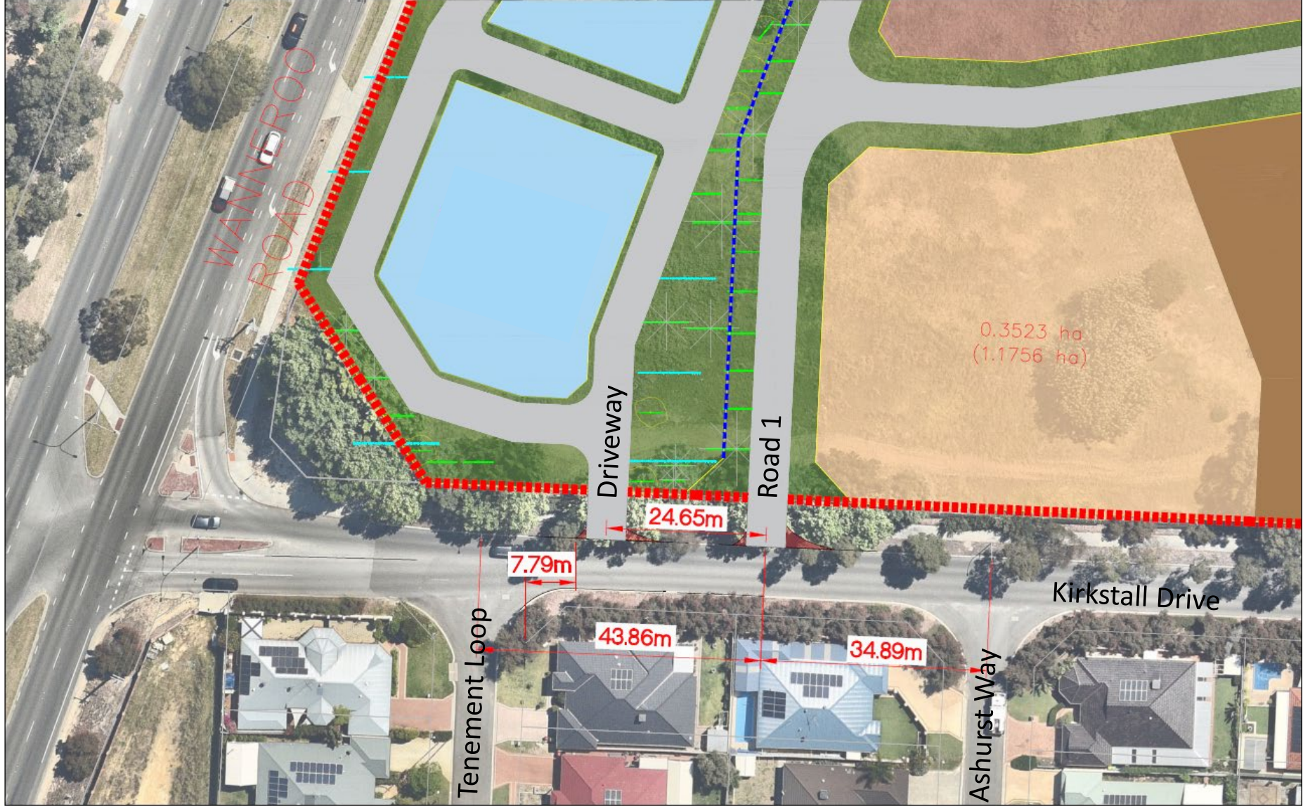
Figure 1: Separation distances between intersections and crossover
